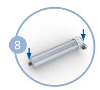
Remove the upper and lower dust caps from each column. There should be a total of two dust caps removed from each column. Make sure there is no dust or debris where the dust caps were located.
