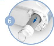
Remove the column completely from the concentrator.
